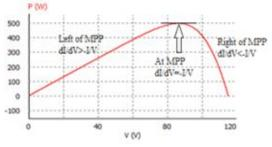
Fig. 2. Operating principle of InC
