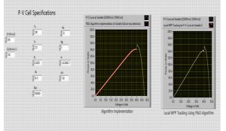
Fig. 8. PV characteristics for a InC algorithm
